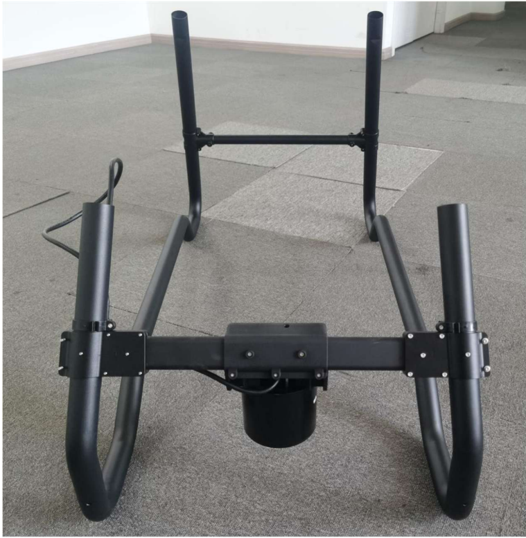
Landing gear module - assembly diagram
